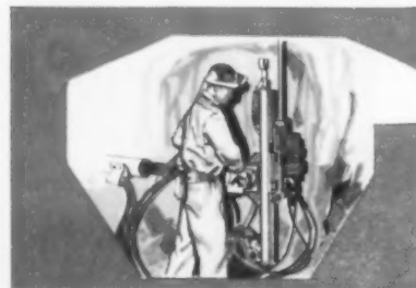
Complete Roof Pinning Machine. Drills the hole, inserts the bolt and tightens the nut.
